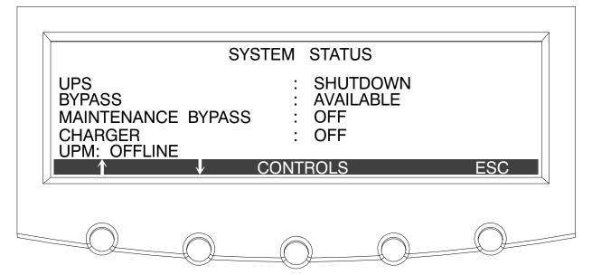
Figure 7-5. Typical System Status Screen
